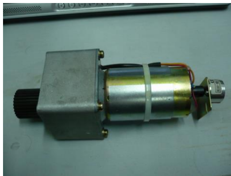
Figure 4.17 DC Motor used to drive the Hip Motion
