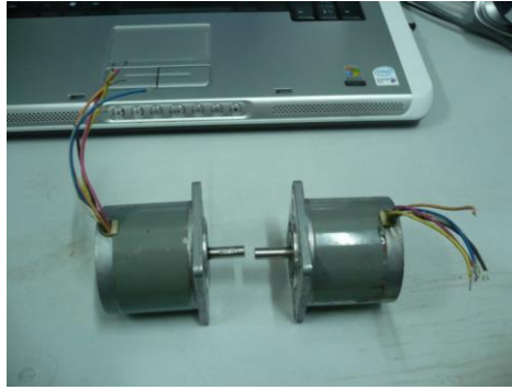
Figure 4.18 Step Motors used to drive the Knee Motion
