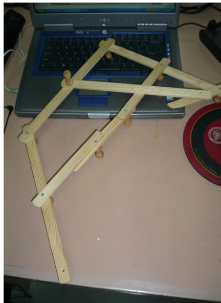
Figure 4.4 Wooden Model of 2-Motor Linkage Design
